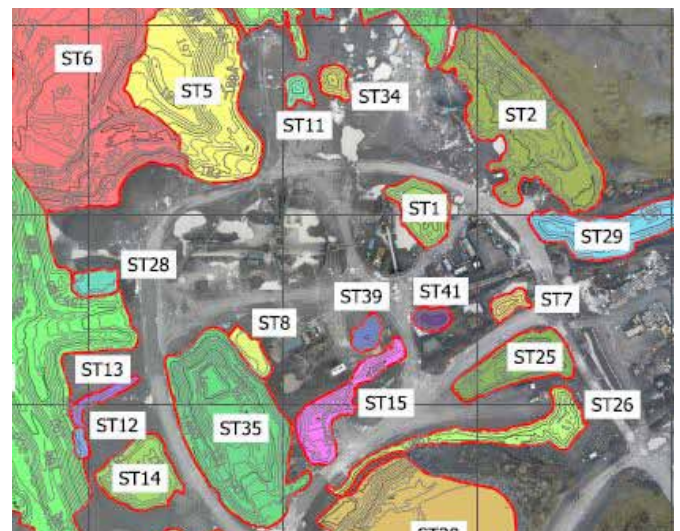
DTM Model (with stockpile identifiers)
